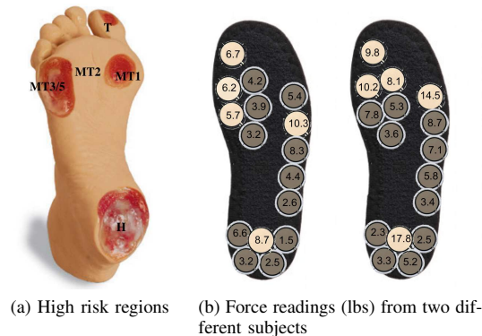
Fig. 3. Medically-important plantar areas and force distribution on custom-made insole with 16 sensors
